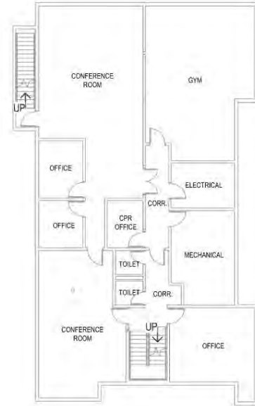
LOWER LEVEL FLOOR PLAN SCALE: 1/16" = 1' -0"
